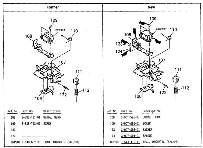
The record/playback head azimuth adjustment is requested due to this change.
