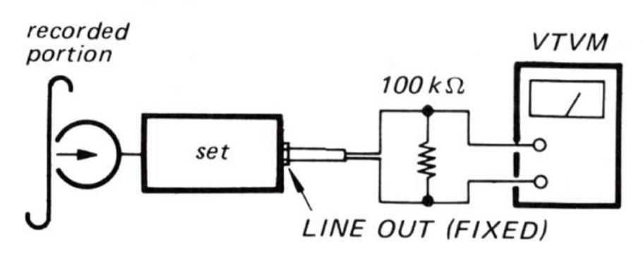
Adjust C128 (L-CH) and C228 (R-CH) to make 1kHz and 10kHz signal output levels equal. If necessary, unsolder portion (a) and solder portion (b).
