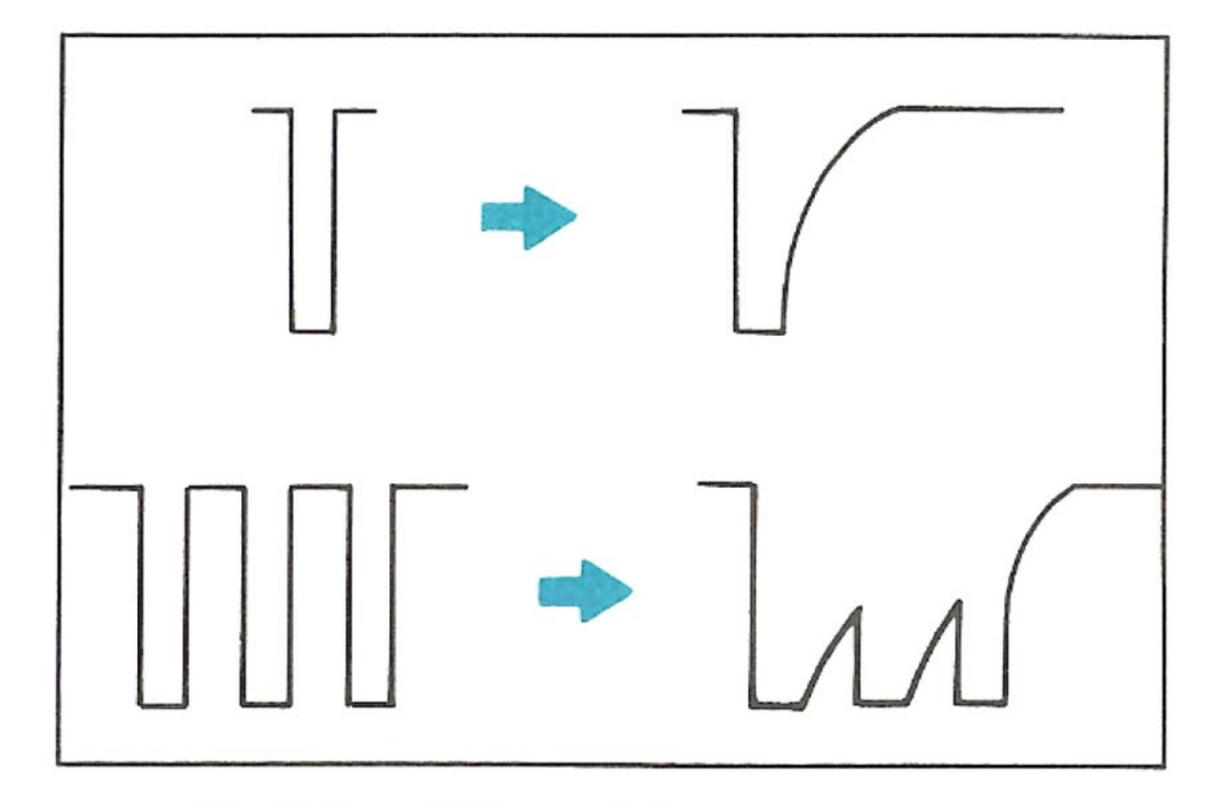
Fig. 1-8. Effect of integrator circuit
