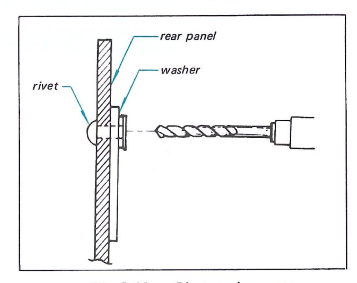
Fig. 2-16. Rivet replacement
