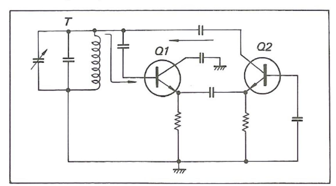
Fig. 1-1. Partial oscillator circuit
