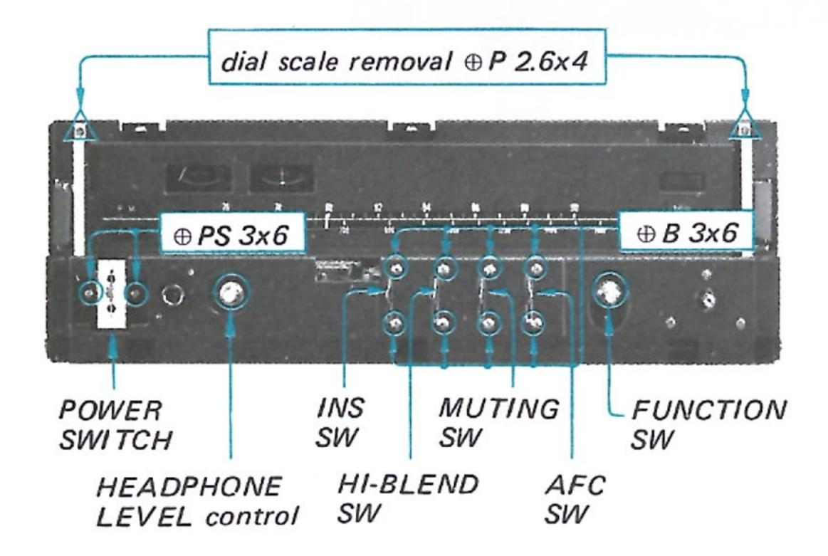
Fig. 2-14. Dial scale, switch and control replacement
