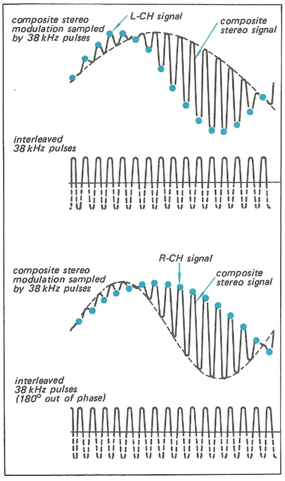
Fig. 1-11. Stereo demodulation operation
