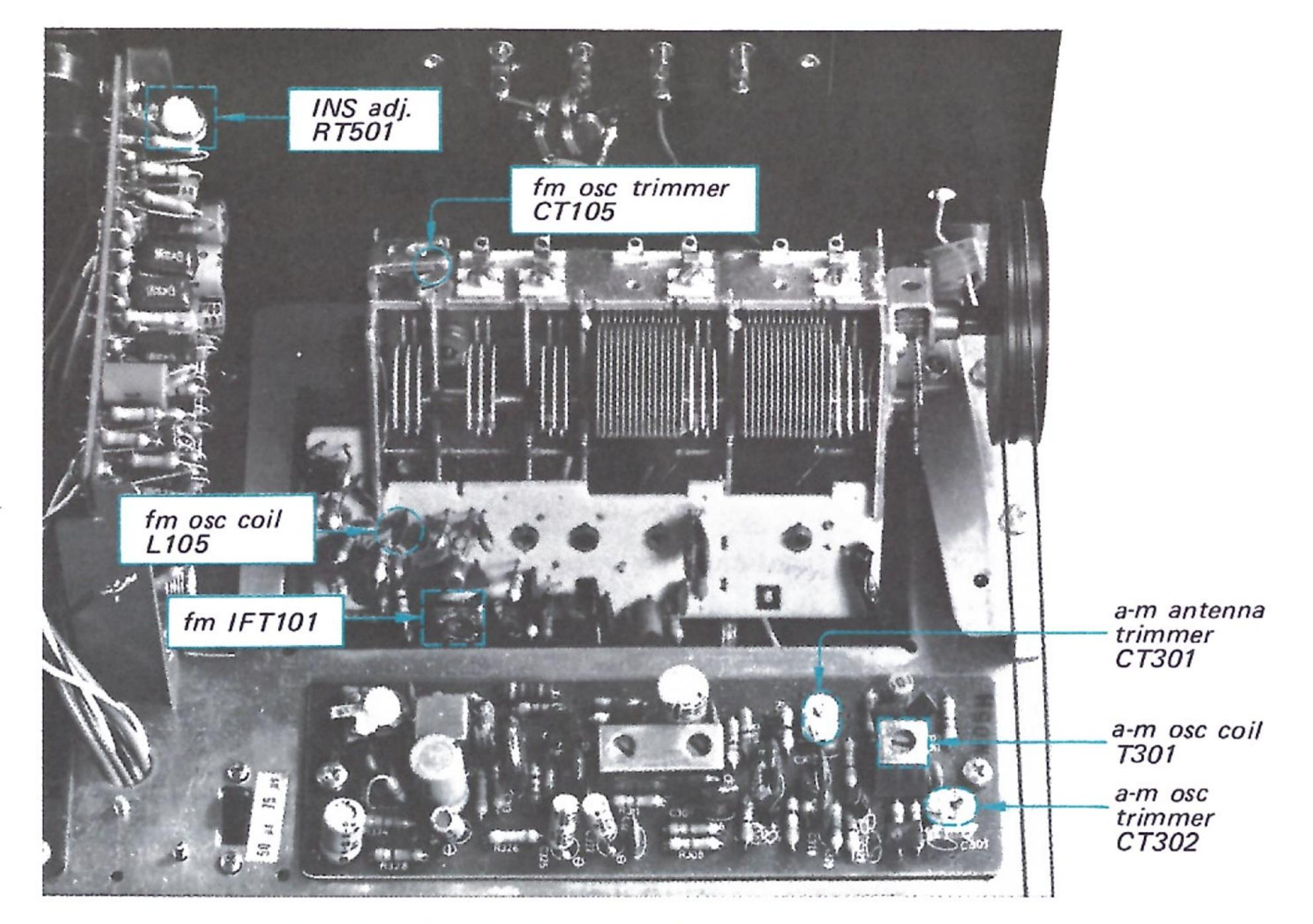
Fig. 3-5. Adjusting parts location
