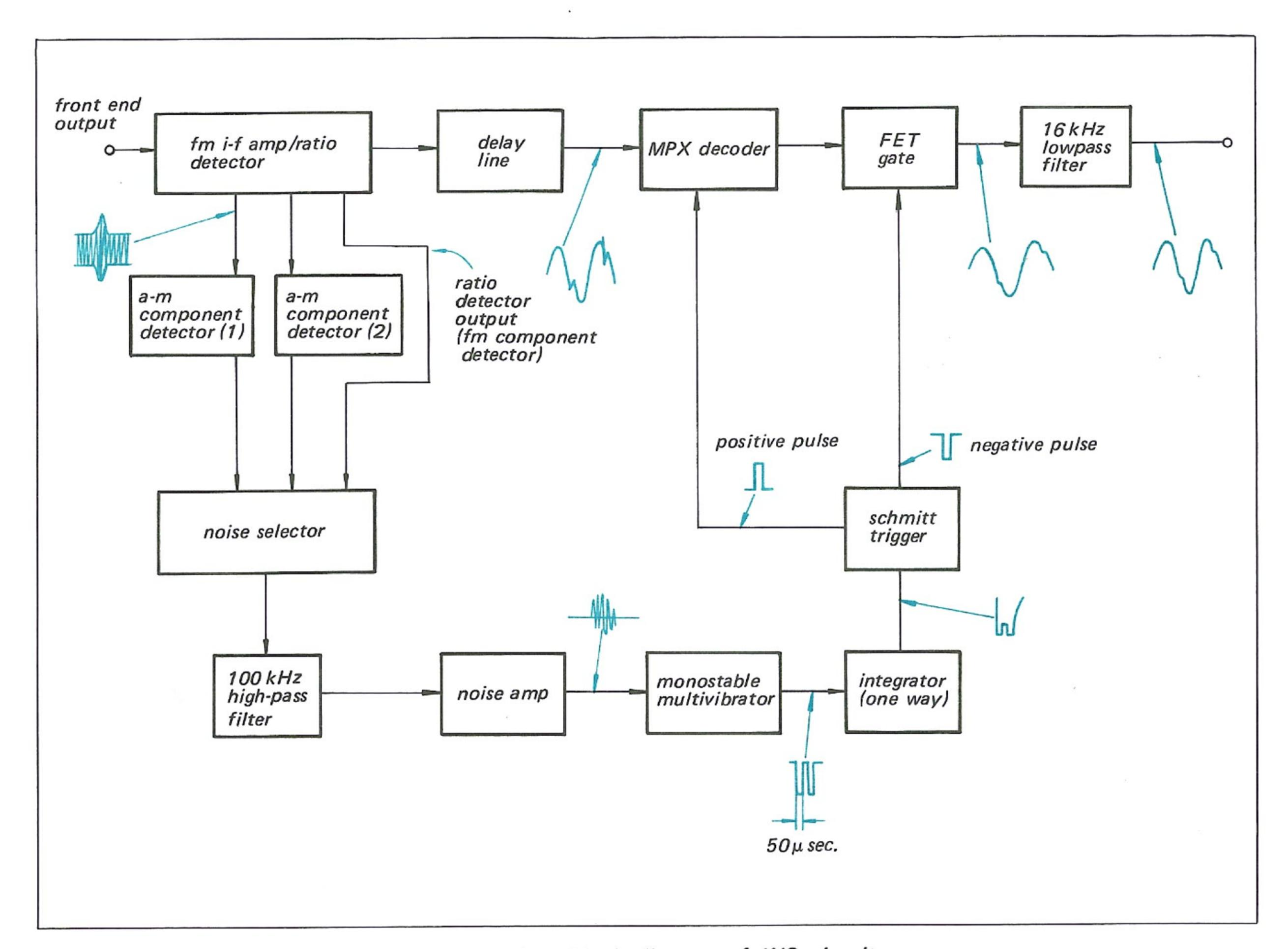
Fig. 1-6. Block diagram of INS circuit
