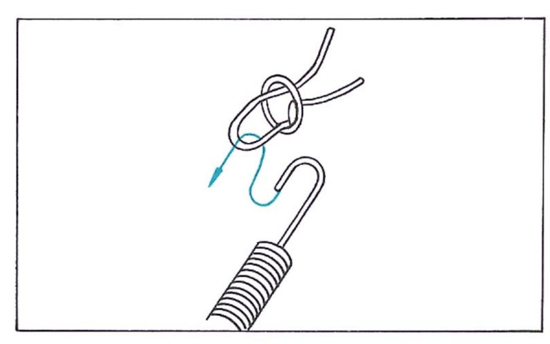
Fig. 2-4. Tying square knot to the coil spring
