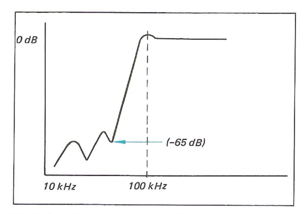
Fig. 1-7. Characteristic of 100 kHz high-pass filter
