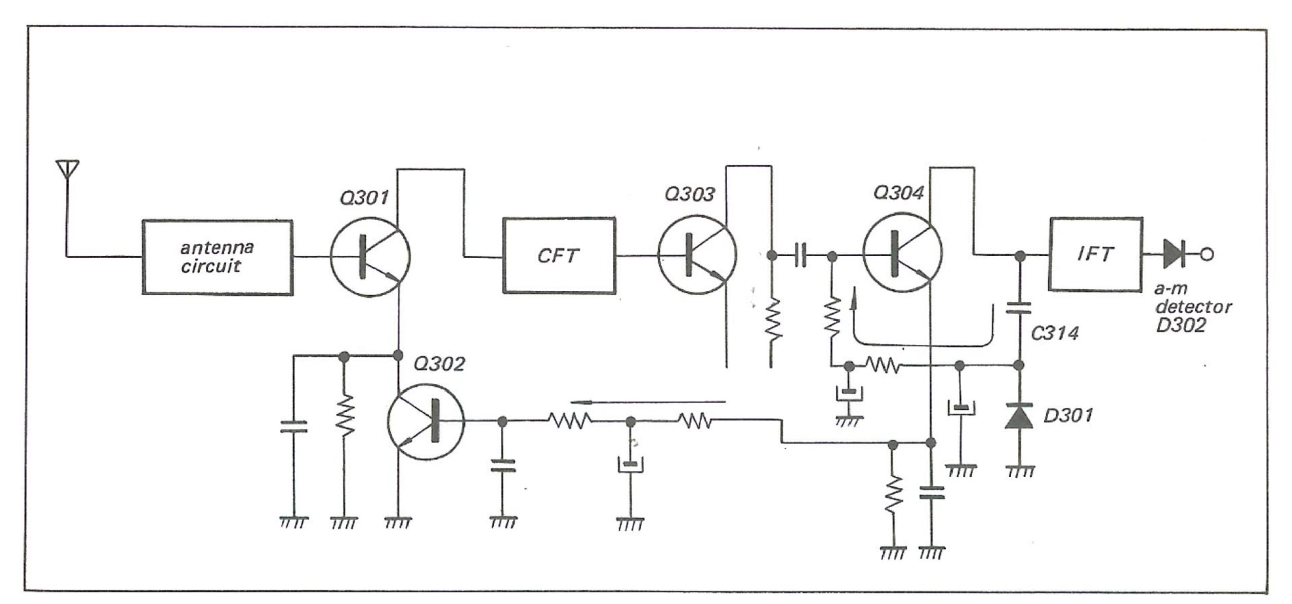
Fig. 1-13. Simplified AGC circuit
