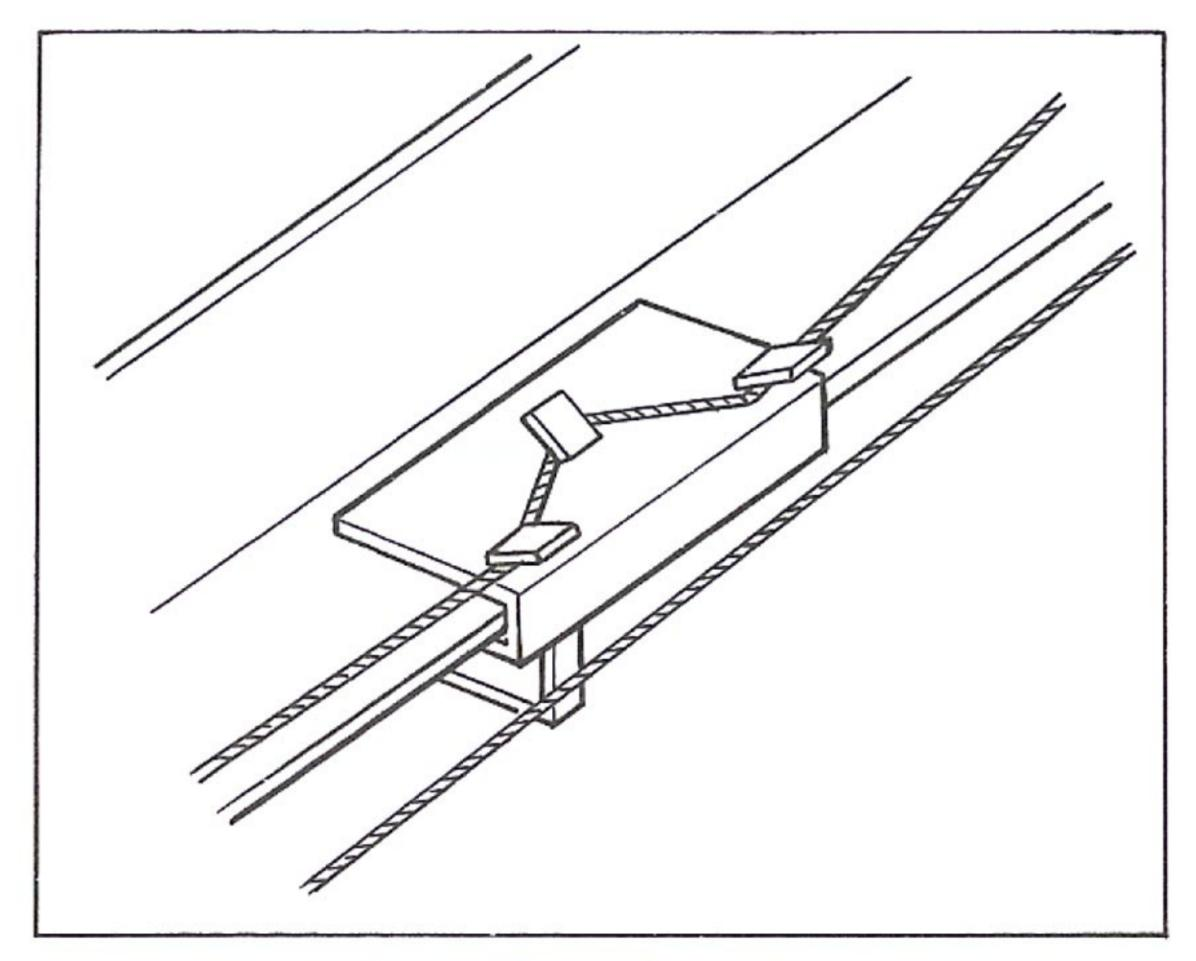
Fig. 2-10. Dial pointer installation
