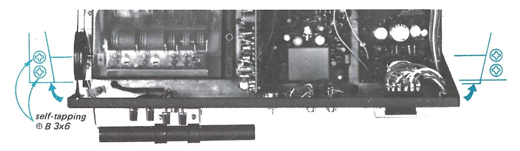
Fig. 2-15. Rear panel removal
