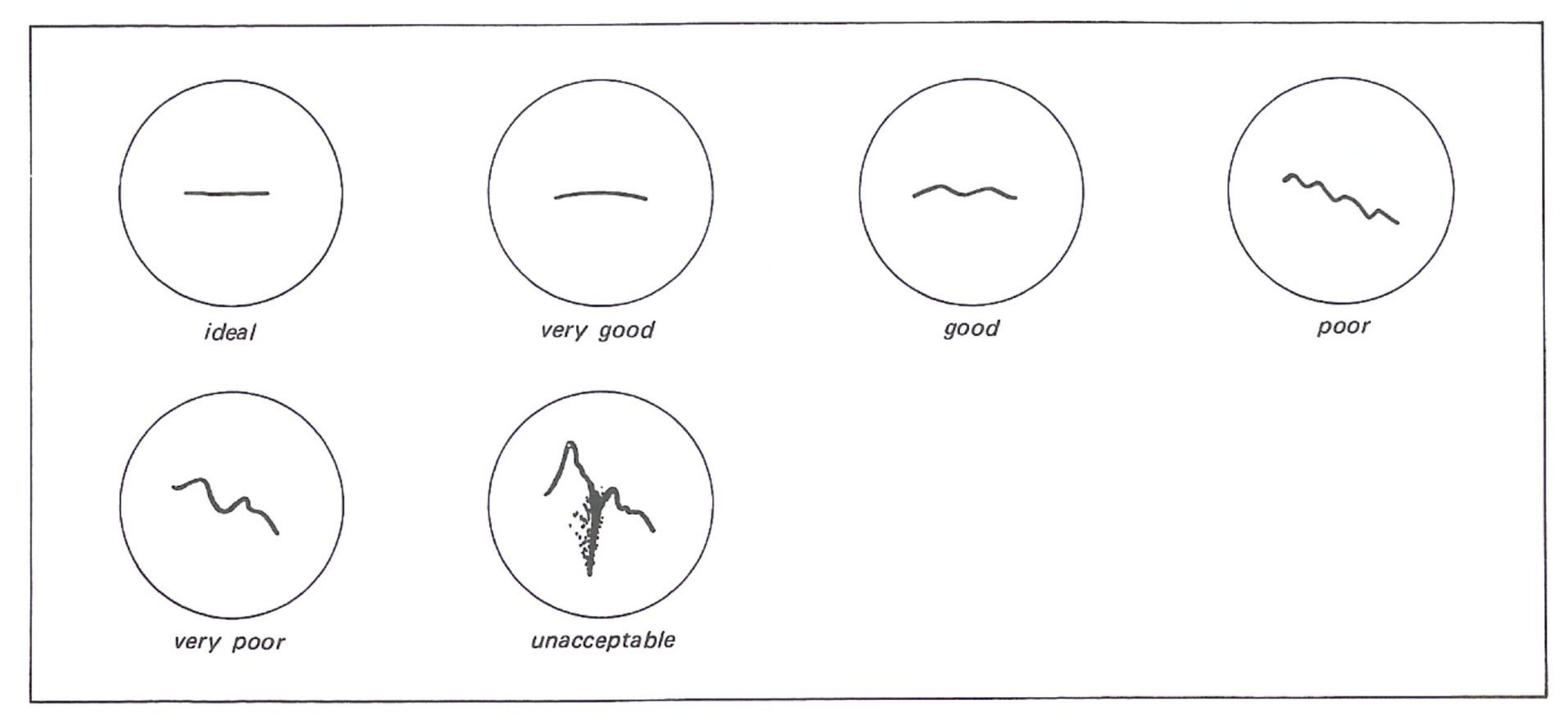
Fig. 1-12. Typical multipath display
