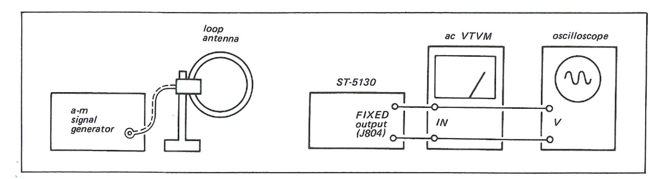
Fig. 3-10. A-m frequency coverage and tracking adjustment
