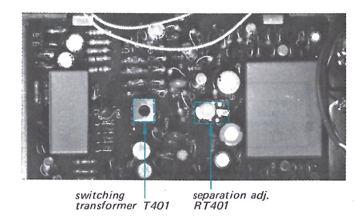
Fig. 3-9. Adjusting parts location
