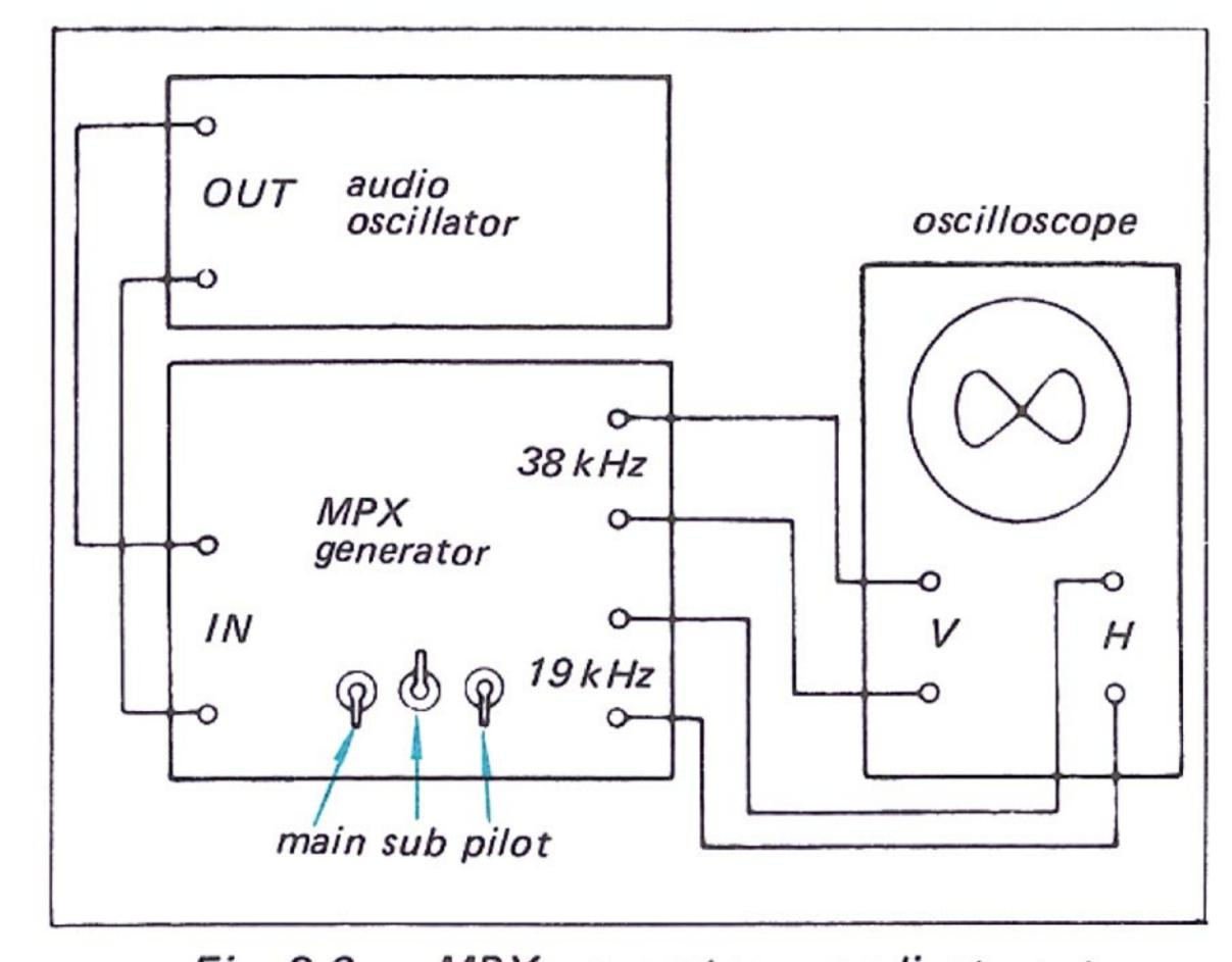
Fig. 3-6. MPX generator preadjustment
