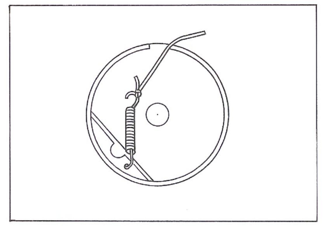
Fig. 2-6. Coil spring installation
