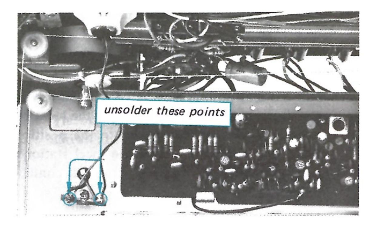
Fig. 2-11. Stereo lamp replacement
