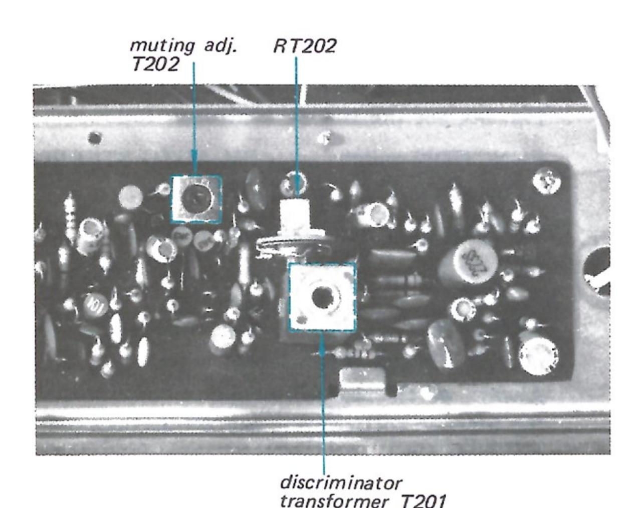
Fig. 3-4. Adjusting parts location
