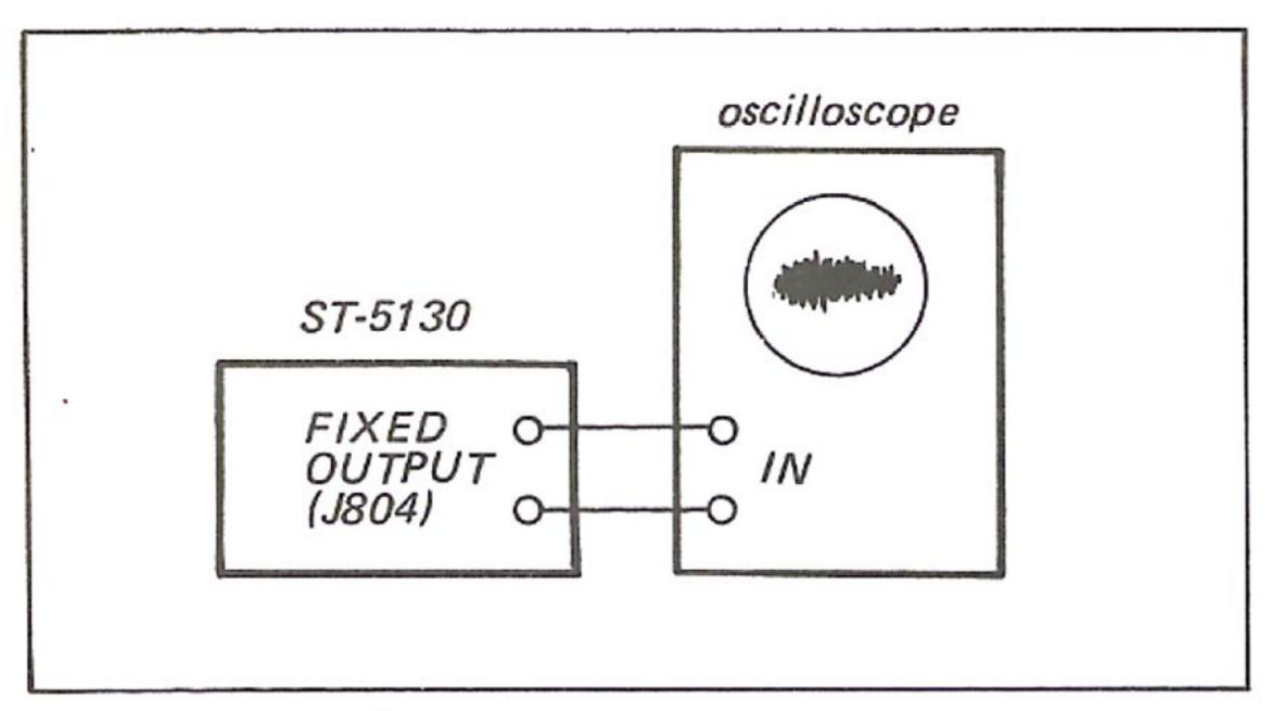
Fig. 3-3. Discriminator alignment test setup
