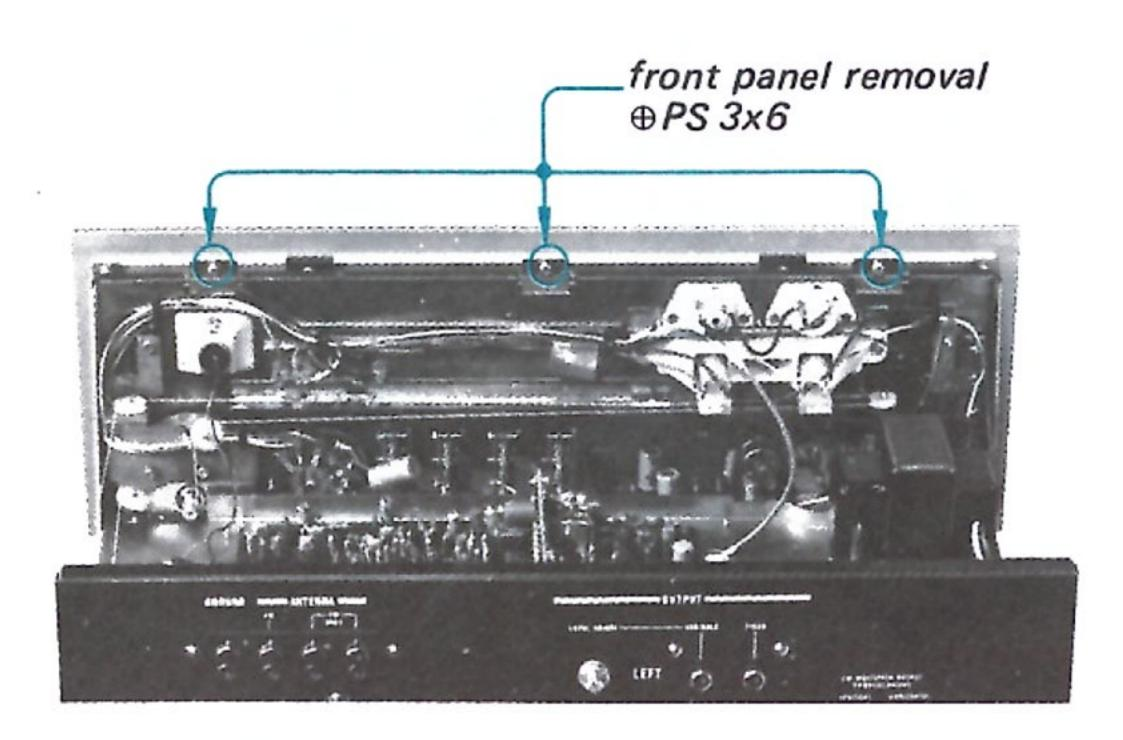
Fig. 2-3. Front panel removal
