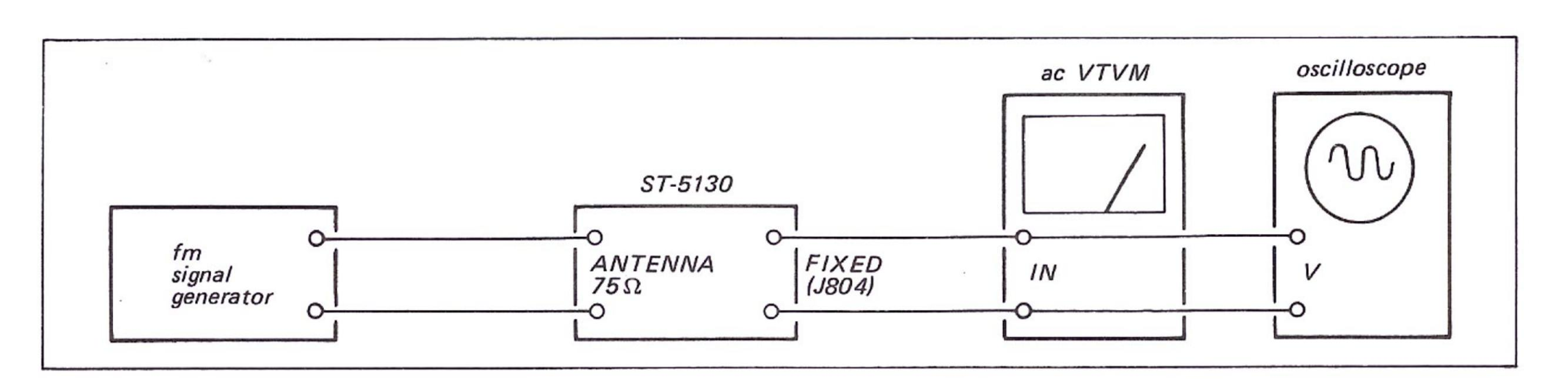
Fig. 3-2. I-f, muting and front-end alignment test setup
