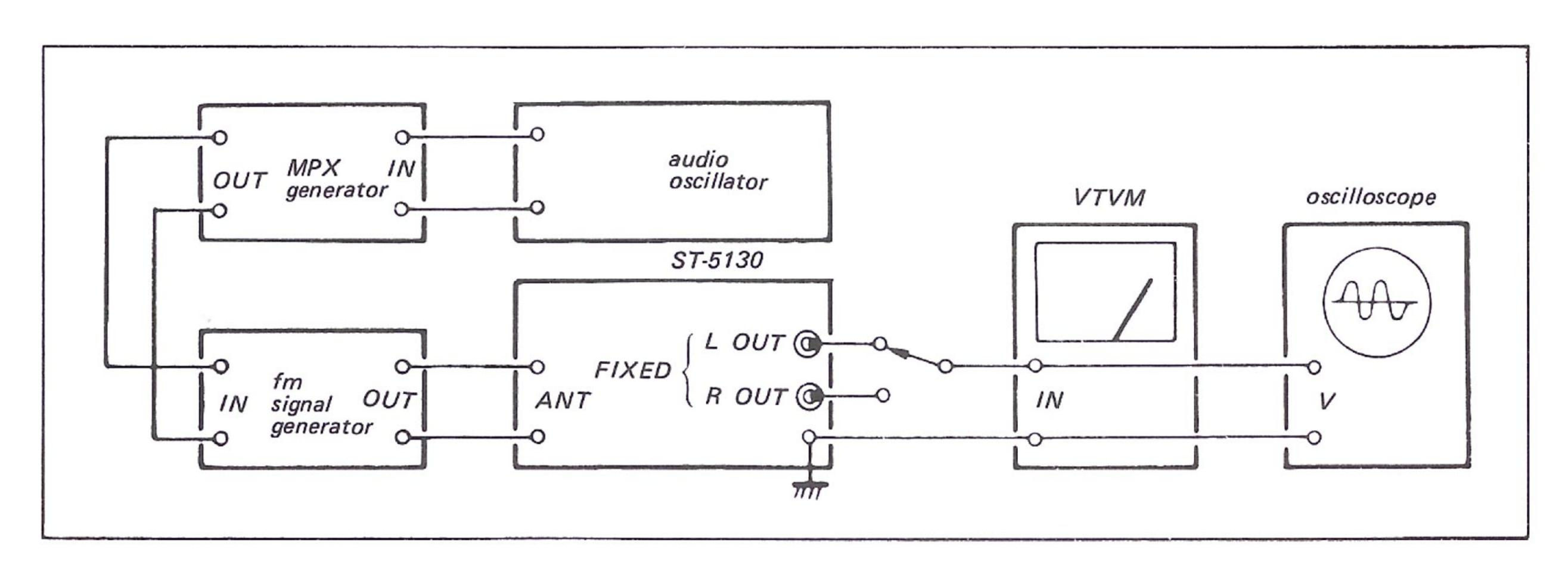
Fig. 3-8. Fm stereo separation adjustment test setup
