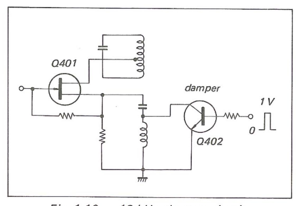
Fig. 1-10. 19 kHz damper circuit
