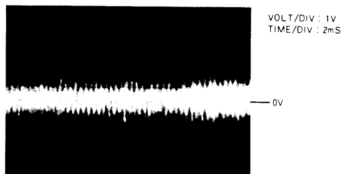
high tracking gain (higher fundamental wave than for low gain)
