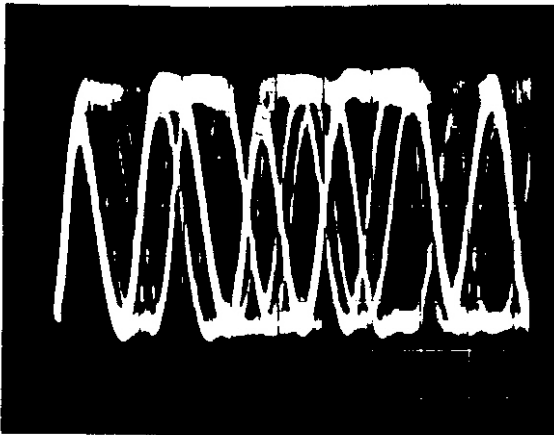
Normal RFO in-between songs 1.2Vp-p Time base = 0.5usec/div.
