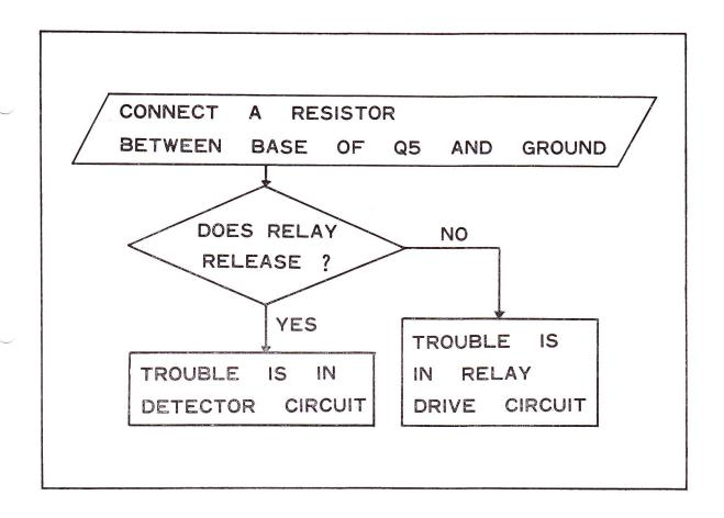
CONNECT A 50K $\Omega$  RESISTOR BETWEEN THE BASE OF Q-5 AND GROUND. IF THE RELAY OPENS AND DISCONNECTS THE SPEAKERS, THEN THE FAILURE IS IN THE DETECTIVE CIRCUITS. IF THE RELAY DOES NOT OPEN, THEN THE RELAY DRIVE CIRCUIT IS DEFECTIVE.
