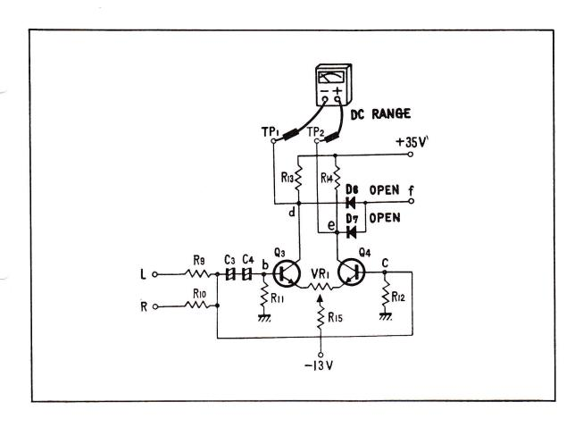
TO CHECK THE D.C. VOLTAGE DETECTION CIRCUIT, CONNECT A MULTIMETER SET FOR D.C. VOLTS BETWEEN TP-1 AND TP-2. TURN VR-1 IN BOTH DIRECTIONS.
