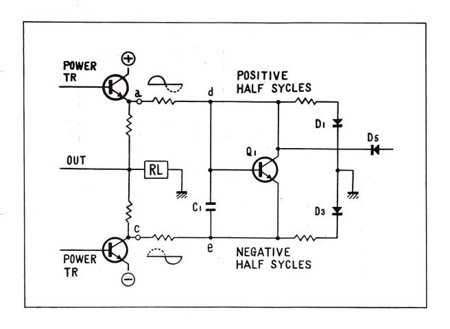
11. THE OUTPUT SIGNAL TO THE SPEAKER IS DEVELOPED ACROSS THE TWO EMITTER RESISTORS CONNECTED AT POINTS "a" "b" AND "c". SINCE WE ARE USING A CLASS "b" PUSH-PULL AMPLIFIER, THE "a" SIDE OF THE AMP HANDLES THE POSITIVE COMPONENTS OF THE SIGNAL BEING AMPLIFIED AND THE "c" SIDE HANDLES THE NEGATIVE.
