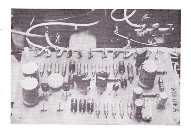
THE MAIN PURPOSE OF HAVING PROTECTION CIRCUITS IN AUDIO EQUIPMENT IS TO PROTECT THE POWER TRANSISTORS IN THE MAIN AMPLIFIER. HOWEVER, IN THE CASE OF OUTPUT CAPACITOR LESS (O.C.L.) MAIN AMPLIFIER CIRCUITS, LOUDSPEAKERS ARE DIRECTLY COUPLED TO THE AMPLIFIER. FOR THIS REASON WE MUST ALSO PROTECT THE SPEAKERS.
