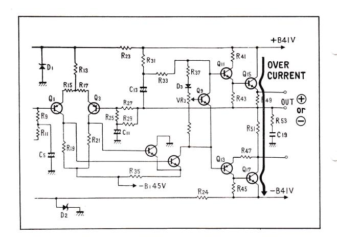
IF A POWER TRANSISTOR SHORTS IN THE MAIN AMP IT WILL UNBALANCE THE AMPLIFIER AND A D.C. VOLTAGE WILL APPEAR ACROSS THE OUTPUT TERMINALS. ALSO, EXCESSIVE CURRENT WILL FLOW THRU THE TRANSISTORS TO GROUND.
