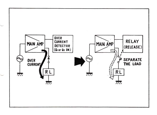
WHEN AN EXCESSIVE CURRENT FLOWS THRU THE LOAD VIA THE MAIN AMP, THE EXCESSIVE CURRENT SENSOR ACUATES THE RELAY AND DISCONNECTS THE LOAD FROM THE AMPLIFIER. NO EXCESS CURRENT WILL FLOW THRU THE POWER STAGE.
