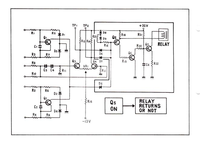
HOWEVER, IF THE MUTING ACTION IS NORMAL, THAT IS IF THE RELAY OPERATES APPROXIMATELY FIVE SECONDS AFTER TURN ON, WE CAN VERIFY NORMAL OPERATION OF Q-5, Q-6 AND Q-7 AND POSSIBLE FAILURE IN THE DETECTION SIDE Q-1 THRU Q-4.
