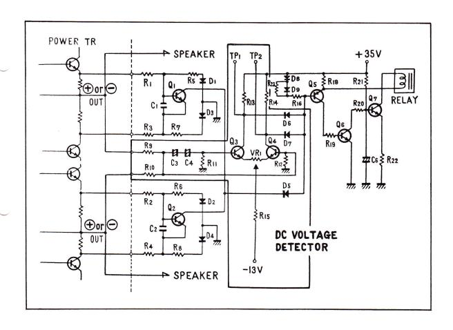
IF ANY D.C. VOLTAGE IS PRESENT AT THE OUTPUT TERMINALS OF THE AMPLIFIER, THE RELAY WILL REMAIN OPEN. UNTIL THE PROBLEM IS CORRECTED, SPEAKERS REMAIN DISCONNECTED SO NO DAMAGE IS POSSIBLE.
