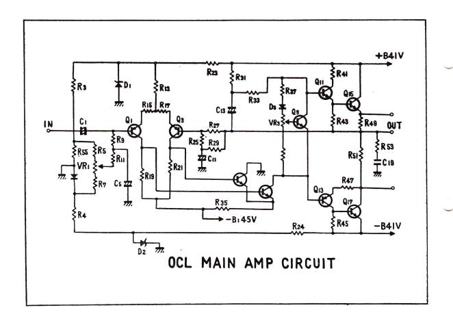
IN ORDER TO MEET THESE REQUIREMENTS, WE DESIGNED A CIRCUIT THAT WOULD DETECT A DEFECTIVE MAIN AMPLIFIER BY SENSING IF THERE IS A D.C. VOLTAGE PRESENT AT THE SPEAKER TERMINALS. THIS ALSO SENSES EXCESSIVE CURRENT IN THE OUTPUT STAGE.
