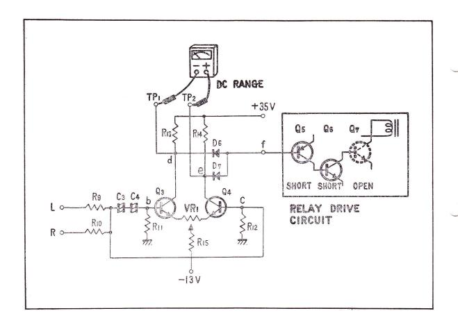
IF BALANCE CANNOT BE OBTAINED BY ADJUSTING VR-1, THEN THE D.C. VOLTAGE DETECTION CIRCUIT MUST BE DEFECTIVE. ALSO, IF THE RELAY DOES NOT WORK EVEN THOUGH THE CIRCUIT IS BALANCED, THEN THE RELAY DRIVE CIRCUIT MAY BE DEFECTIVE. POSSIBLE CAUSES MAY BE A SHORT IN Q-5 OR Q-6 OR AN OPEN IN Q-7.
