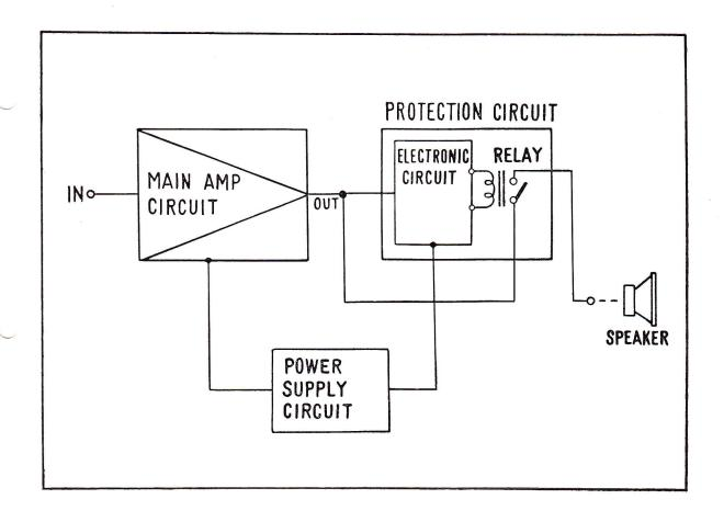
IN PIONEER O.C.L. MAIN AMP'S A "CUT OFF LOAD SYSTEM" IS EMPLOYED. THIS IS AN ELECTRIC SENSING CIRCUIT AND RELAY WHICH DISCONNECTS THE SPEAKERS FROM THE AMP WHENEVER THE AMPLIFIER OR SPEAKER MAY BE DEFECTIVE.
