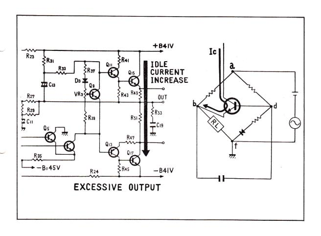
IF THE POTENTIAL OF POINT "a" INCREASES BECAUSE OF EXCESSIVE OUTPUT OR HIGH IDLE CURRENT OR IMPROPER BIAS, EXCESSIVE CURRENT WILL FLOW THRU THE POWER TRANSISTORS CAUSING A LARGER VOLTAGE DROP ACROSS THE EMITTER RESISTORS. BECAUSE OF THIS, THE POTENTIAL AT POINT "b" WILL INCREASE CAUSING AN IMBALANCE OF THE BRIDGE CIRCUIT, WHICH WILL ACUATE THE PROTECTION RELAY.
