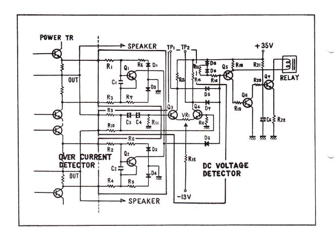
8. WE CAN DIVIDE THE PROTECTION UNIT INTO THREE SECTIONS, CONSISTING OF TRANSISTORS Q-1 AND Q-2, Q-3 AND Q-4 AND Q-5, Q-6, Q-7.
