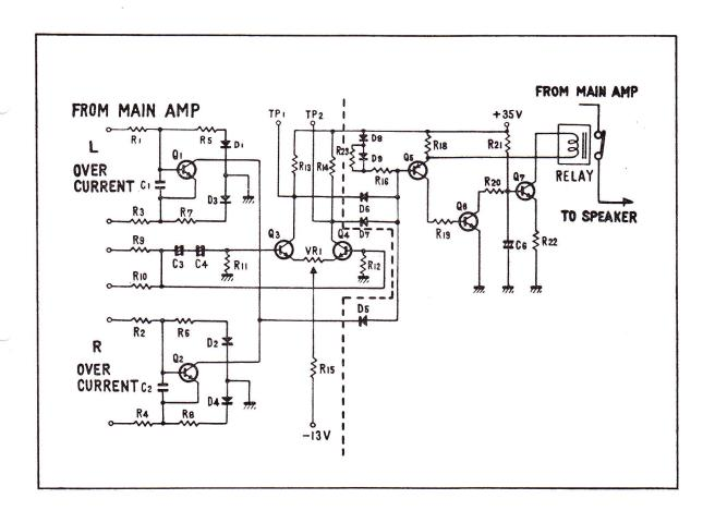
WHENEVER THE RELAY IS NOT ENERGIZED, THE CURRENT DETECTION CIRCUIT, CONSISTING OF Q-1 AND Q-2 WILL TURN OFF WHICH INCREASE THE BASE POTENTIAL AT Q-5. THIS TURNS OFF Q-5 AND Q-6. Q-7 WILL TURN ON, ENERGIZING THE RELAY WHICH CONNECTS THE SPEAKERS AND AMP. IF THE ORIGINAL PROBLEM WHICH CAUSED THE RELAY TO OPEN IN THE FIRST PLACE STILL EXSISTS THEN THE CIRCUIT WILL CYCLE ON AND OFF UNTIL THE PROBLEM IS CORRECTED.
