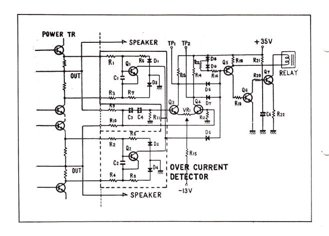
HERE WE WILL EXPLAIN IN DETAIL HOW EACH OF THE CIRCUITS WORK. WE WILL START WITH THE CURRENT OVERLOAD SENSING CIRCUIT. AS YOU CAN SEE Q-1 AND Q-2 ARE THE SAME. ONE FOR EACH CHANNEL, SO WE WILL EXPLAIN ONLY ONE SIDE.
