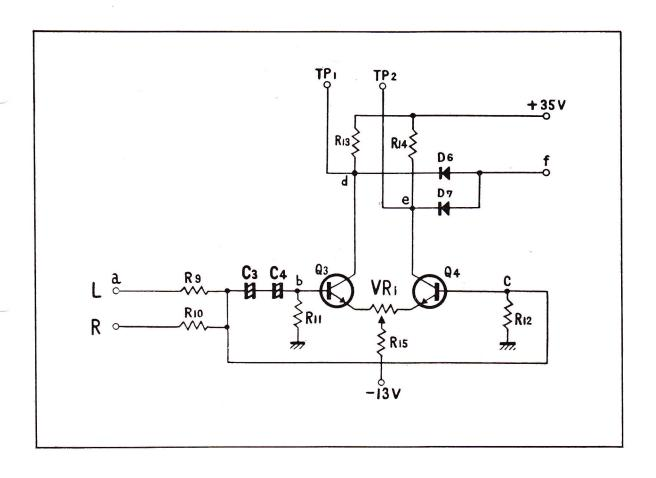
AS CAN BE SEEN IN THE SCHEMATIC, THE BASES OF Q-3 AND Q-4 ARE CONNECTED TO CAPACITORS C-3 AND C-4. THESE CAPACITORS ARE CONNECTED IN SERIES. BY ITS DESIGN, A DIFFERENTIAL AMPLIFIER ONLY HAS OUTPUT WITH A DIFFERENCE IN INPUT. SINCE WE NEED SOME METHOD OF SENSING THIS DIFFERENCE, NECESSARY FOR OPERATION, WE HAVE INSTALLED THESE CAPACITORS AT THIS POINT IN THE CIRCUIT.
