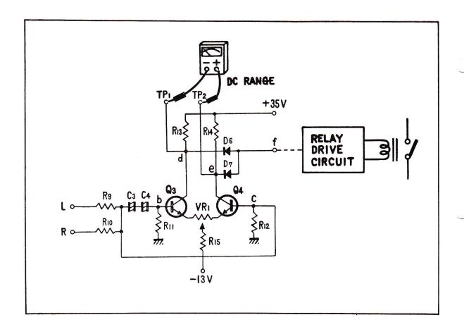
WHEN YOU TURN VR-1 CLOCKWISE AND COUNTER-CLOCKWISE, IF THE CIRCUIT IS NORMAL, AT SOME POINT, IN THE ROTATION, YOU WILL GET A VOLTAGE READING BETWEEN TP-1 AND TP-2. ALSO, THE RELAY SHOULD OPEN. IF WHEN YOU FIRST CHECK THE VOLTAGE READING AND ROTATING VR-1 HAS NO AFFECT, THEN Q-3 OR Q-4 MAY BE DEFECTIVE.
