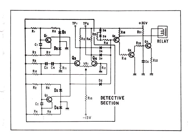
POSSIBLE CAUSES FOR TEMPERATURE SENSITIVITY IN THE DETECTION CIRCUIT ARE AN UNBALANCING OF THE DIFFERENTIAL AMPLIFIER CAUSED BY Q-3, Q-4 OR D-1 THRU D-4.
