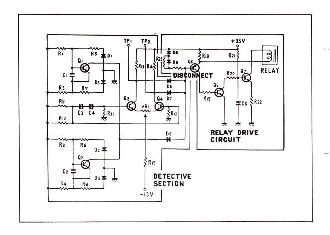
TO TELL WHICH SIDE HAS THE PROBLEM YOU MUST SEPARATE THE RELAY DRIVE CIRCUIT FROM THE DETECTION CIRCUIT. THE RELAY ITSELF WILL GIVE YOU A CLUE AS TO WHICH SIDE IS BAD.
