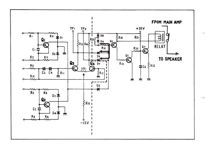
NEXT WE'LL SEE HOW THE RELAY DRIVE CIRCUIT OPERATES. IF COLLECTOR CURRENT FLOWS IN Q-1, Q-2, Q-3, OR Q-4 THE DIODE CONNECTED TO THEIR COLLECTOR IS FORWARD BIASED AND THIS CAUSES A VOLTAGE DROP ACROSS R-16. THIS VOLTAGE DROP WILL DECREASE THE POTENTIAL AT THE BASE OF Q-5 BY AN AMOUNT EQUAL TO THE DROP ACROSS R-16.
