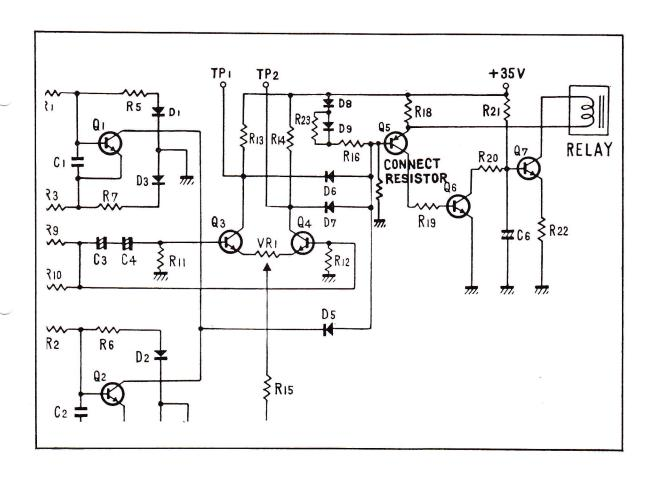
39. TO CHECK THE RELAY OPERATION WE CAN TURN Q-5 ON BY CONNECTING A 50K  $\!\Omega$  1/2W RESISTOR FROM THE BASE OF Q-5 TO GROUND.
