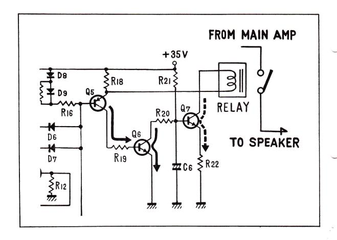
26. WHEN COLLECTOR CURRENT FLOWS THRU Q-6 A LARGE VOLTAGE DROP WILL APPEAR ACROSS R-21, CAUSING A BASE VOLTAGE DROP AT Q-7. THIS WILL CUT-OFF COLLECTOR CURRENT WHICH WILL DISCONNECT THE AMPLIFIER FROM THE SPEAKERS.
