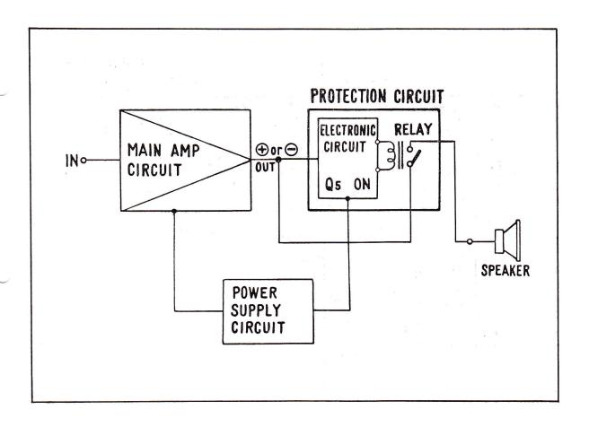
23. IN THIS MANNER, WHENEVER A POSITIVE OR NAGATIVE VOLTAGE IS PRESENT AT THE OUTPUT TERMINALS, Q-5 WILL CONDUCT, ACTUATING THE RELAY TO DISCONNECT THE SPEAKERS.
