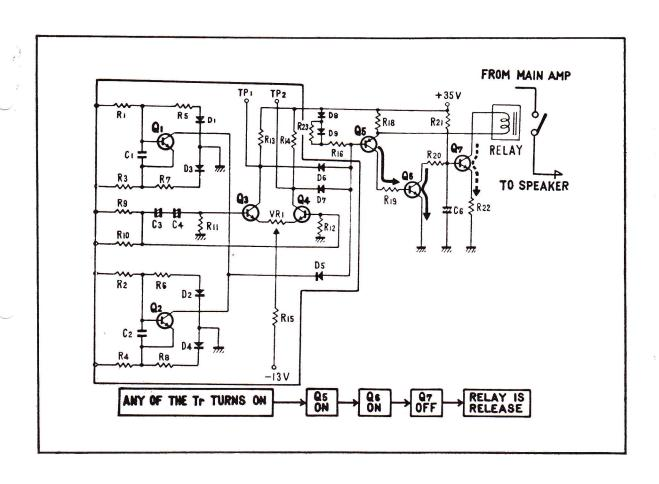
NOW WE WILL CONSIDER THE PROTECTION UNIT ITSELF: IF FOR ANY REASON, Q-1, Q-2, Q-3, OR Q-4 TURNS ON. THEN THIS WILL LOWER THE BASE POTENTIAL OF Q-5 WHICH WILL TURN OFF THE RELAY BY TURNING ON Q-5 AND Q-6 AND TURNING OFF Q-7.
