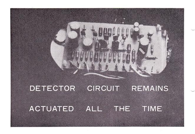
NOW WE WILL CONSIDER THE PROBLEM OF THE PROTECTION CIRCUIT REMAINING ACTUATED ALL THE TIME. THIS IS PROBABLY CAUSED BY D.C. VOLTAGE AT THE OUTPUT TERMINALS.
