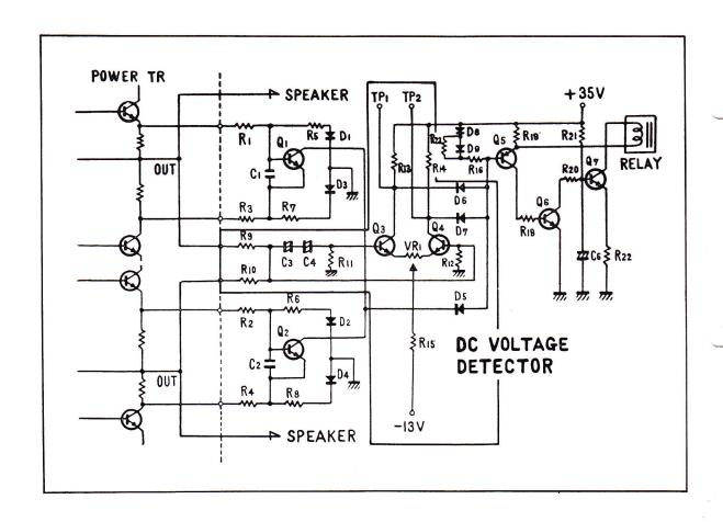
MOST LIKELY THIS IS CAUSED BY AN UNBALANCED DIFFERENTIAL AMP IN D.C. DETECTION CIRCUIT.
