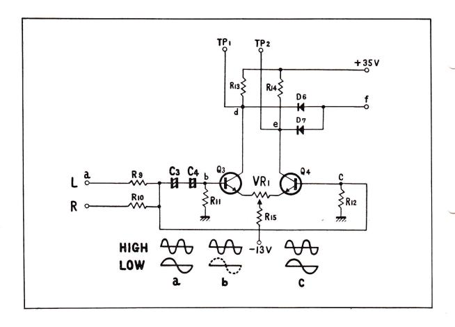
THE REACTANCE OF C-3 AND C-4 MAY BE DISREGARDED AT ANY FREQUENCY OVER A FEW HERTZ. SINCE THE BASES OF Q-3 AND Q-4 ARE FED THE SAME SIGNAL, THERE IS NO DIFFERENCE SIGNAL PRESENT AND NO OUTPUT. HOWEVER, FOR SIGNALS BELOW A FEW HERTZ OR DIRECT CURRENT THE REACTANCE OF C-3 AND C-4 CANNOT BE DISREGARDED. THEREFORE, A DIFFERENCE SIGNAL WILL BE PRESENT BETWEEN THE BASES OF Q-3 AND Q-4. THIS WILL CAUSE OPERATION OF THE RELAY.
