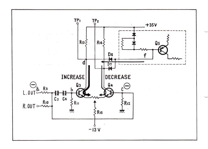
IF NEGATIVE VOLTAGE IS APPLIED TO POINT "a", THE COLLECTOR CURRENT OF Q-4 WILL DECREASE IN PROPORTION TO THE VOLTAGE AT THE BASE, WHILE THE COLLECTOR CURRENT OF Q-3 WILL INCREASE. THIS INCREASE WILL CAUSE THE POTENTIAL AT POINT "d" TO DECREASE IN INVERSE PROPORTION TO THE COLLECTOR CURRENT AT Q-3. AGAIN THIS WILL FORWARD BIAS THE DIODE D-6 WHICH WILL REDUCE POTENTIAL AT POINT "f", TURNING Q-5 ON AND OPERATING THE RELAY.
