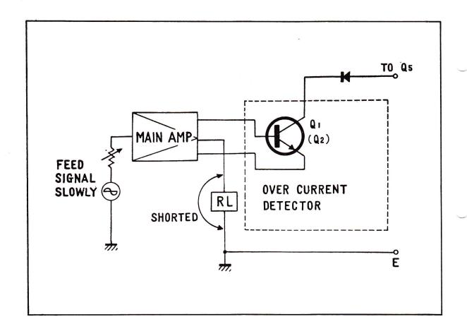
TO CHECK THE EXCESSIVE CURRENT DETECTION CIRCUIT INSURE THAT NO SIGNAL IS FED INTO THE AMPLIFIER. SHORT CIRCUIT BOTH OUTPUT TERMINALS AND VERY SLOWLY FEED A SIGNAL TO THE INPUT. YOU SHOULD BE CHECKING WITH YOUR MULTIMETER THAT THE COLLECTOR VOLTAGE OF Q-1 AND Q-2 DECREASES QUICKLY AS THEY TURN ON.
