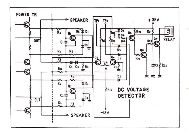
NOW WE WILL CONSIDER THE OPERATION OF THE D.C. VOLTAGE DETECTION CIRCUIT. THIS CIRCUIT IS COMPOSED OF TRANSISTORS Q-3 AND Q-4. IT IS DESIGNED TO OPERATE THE PROTECTION RELAY WHENEVER THERE IS D.C. VOLTAGE PRESENT AT THE SPEAKER TERMINALS. Q-3 AND Q-4 ARE A MATCHED PAIR FORMING A DIFFERENTIAL AMPLIFIER. A BIAS ADJUSTING CIRCUIT IS PROVIDED TO COMPENSATE FOR MINOR CIRCUIT VARIATIONS AND TO BALANCE THE DIFFERENTIAL AMP.
