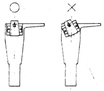
When the cartridge is replaced, refer to page 6 and 7 and adjust stylus tracking force.
