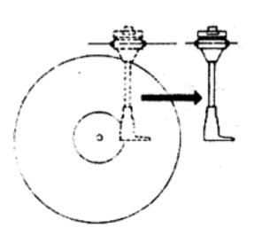
The tonearm is automatically returned to the arm clamp position, and the platter is stopped.
