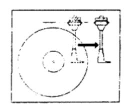
Depress the arm elevation switch to raise the tonearm (temporary stop)
