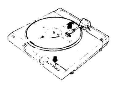
The arm-elevation lamp ▼ should illuminate.
