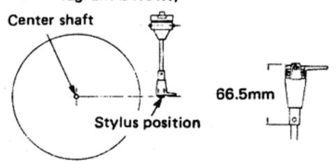
Attach the cartridge to the headshell with the front faces parallel to each other. (If the cartridge is not straight, it may cause the tonearm to operate improperly and/or create distortion.)
