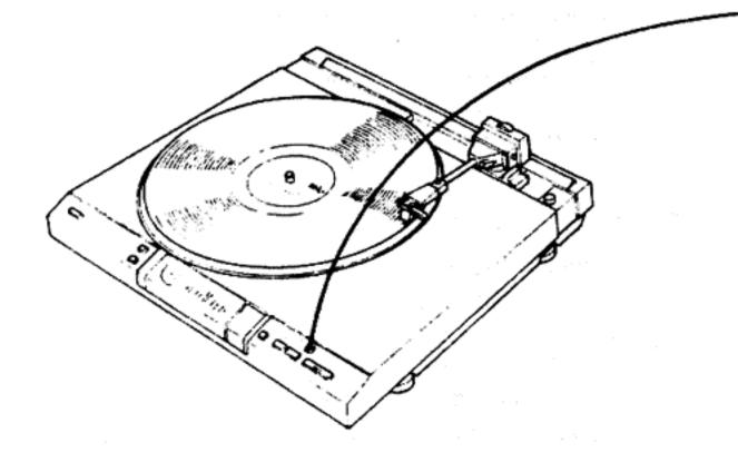
3. Start playback. (Depress the arm-elevation switch)
