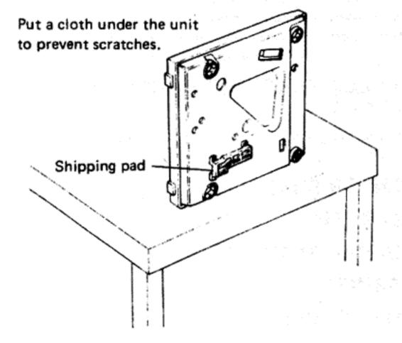
Steady the unit with one hand to prevent it from falling, and using a medium-sized Phillips screwdriver with the other hand, remove the four screws.
