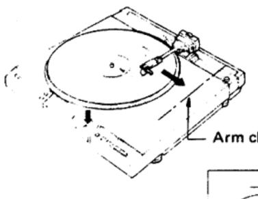
The tonearm will automatically return to the arm clamp position and stop platter rotation.
