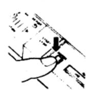
3. Start playback by depressing the playback start/stop switch
