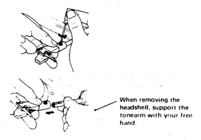
3. Disconnect the lead wires from the cartridge.
