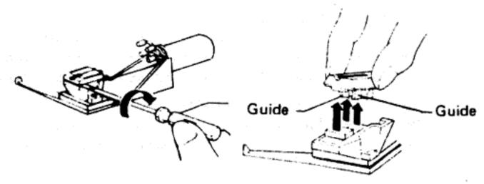
5. Connect the lead wires to the new stylus holder.
