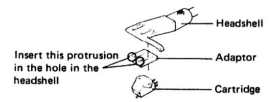
Adjust the position of the headshell cartridge to where the stylus will travel over the exact center of the center shaft. (This is a simple adjustment. Refer to the diagram below.)
