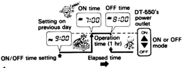
When combined with the tape deck and tuner, the timer can record radio programs unattended.
