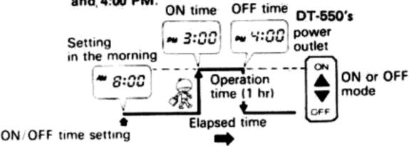
One ON and one OFF time can be set on the timer in a 24-hour period of time.
