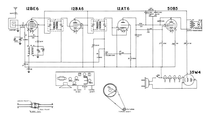
This is a five tube, single band, superheterodyne receiver, incorporating a built-in loop antenna and four inch P.M. type speaker. Tuning range is 540 to 1600 kc, and the receiver is designed for either 117 volt—25-60 cycles A.C. or 117 volt D.C. line operation and consumes approximately 30 watts of power.
