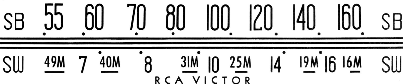
Fig. 7—The Dial Scale drawing shown is a full size reproduction. It can be used as a reference in alignment procedure. (9Y5S)
