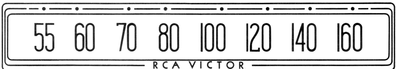
Fig. 1. The Dial Scale drawing shown is a full size reproduction. It can be used as a reference in alignment procedure. (9Y5)
