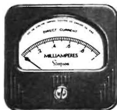
MODELS 127, 137, 147, 157, 2 1/2" RECTANGULAR ACCURACY: 2% SCALE LENGTH: 1-7/8"
