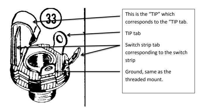
Note the large "U" shape bar, that's the "TIP" bar that connects to the TIP tab. The short straight "strip" is the "Switch Strip" that connects to the "Switch tab". The other tab is ground. This socket's switch replaces the front panel "Push/Pull" RF gain control switch. When properly
