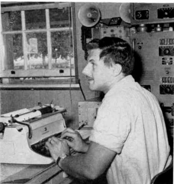
Radioman at Rockaway (N.Y.) USCG Station has hurried look as he nears end of 6-hour duty. Receiver at top of panel continually monitors 2182 kHz and has switch knob removed to prevent accidental switching away from distress channel. (Coast Guard Photo)
