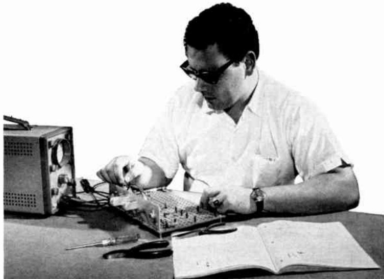
Performing transistor experiments on programmed breadboard—using oscilloscope
