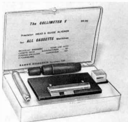
Ramko Research Collimeter II (cartridge) and Collimeter V (cassette) tape head and guide alignment kits are shown above and below, respectively, in plastic cases.
