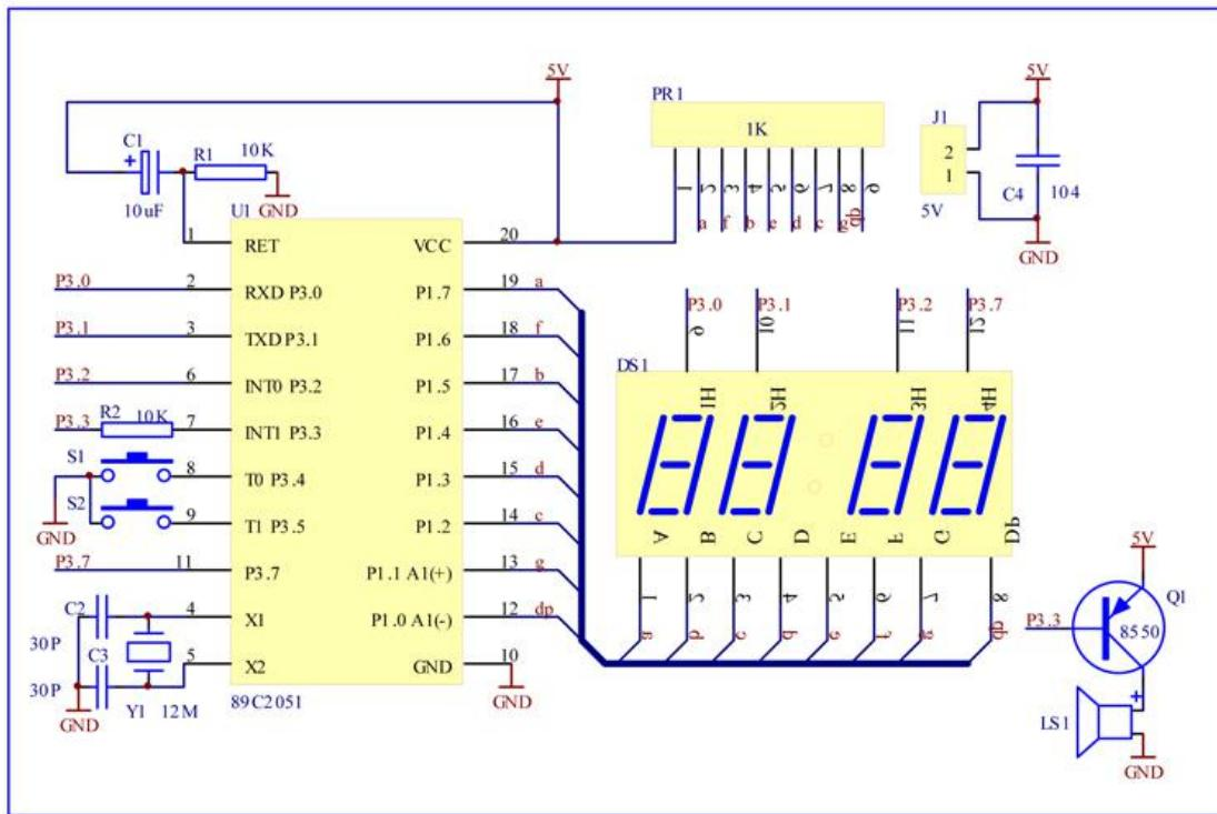
Note: there is direction for PR1 Resistors Packs , there is one side of the word in the direction of the MCU.Pay an attention!!!
