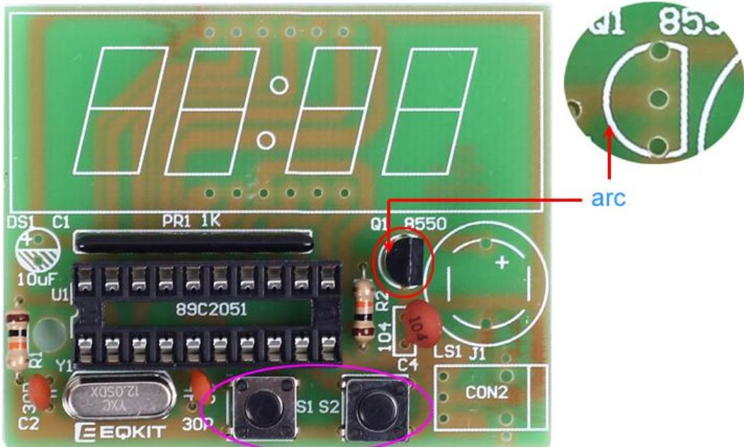
**Step 5: Install 1pcs Power Socket at J1. 1pcs 10uF 25V Electrolytic**
