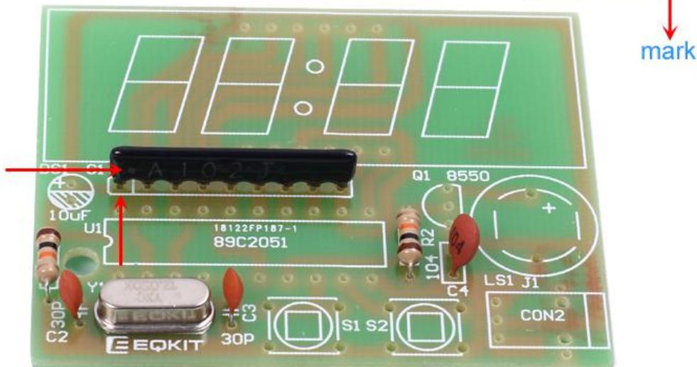
Step 3: Install 1pcs DIP-20 IC Socket at U1 and pay attention to the installation direction. There is a smaller notch on IC Socket and there is a white mark on PCB where the IC Socket can place on. These two marks are corresponding to each other and are used to specify the installation direction of the IC Socket.
