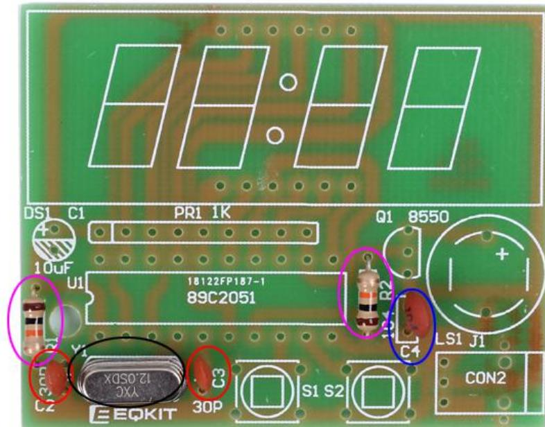
Step 2: Install 1pcs 1Kohm Network Resistor at PR1. Pay attention to the installation direction. There is a smaller dot on one corner of the Network Resistor and there is a white mark on PCB where the Network Resistor can place on. These two marks are corresponding to each other and are used to specify the installation direction of the Network Resistor.
