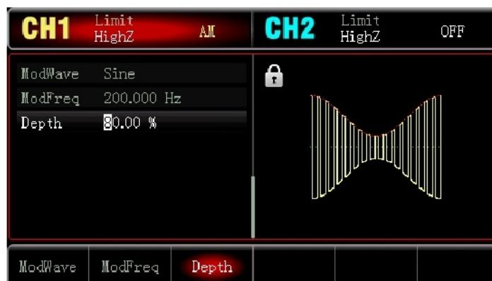
The AM modulation waveform in oscilloscope is shown below:
