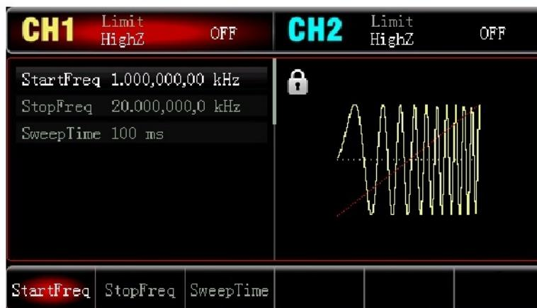
Press **StartFreq** / **StopFreq**, enter 1 by numeric keypad, and select the parameter unit **kHz**.
