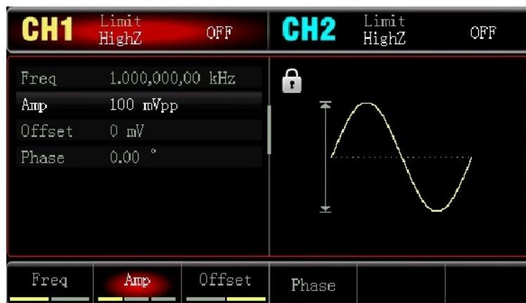
Press **Freq** to set frequency, enter 10 by numeric keypad, and select parameter unit **kHz**.
