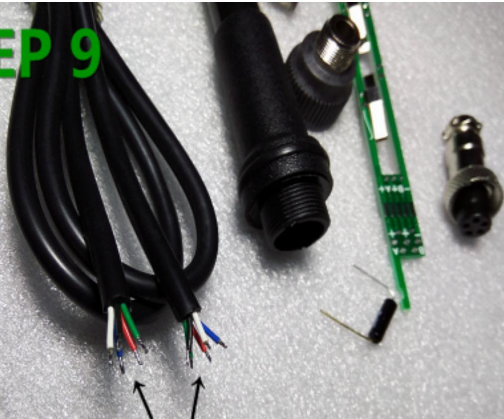
Wire stripping and soldering
