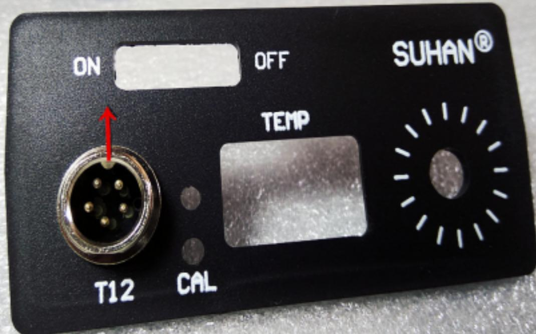
Put the Aviation plug into the front-panel
