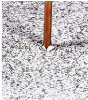
Figure 12-2 (The magnetic field produced by the current in a wire through a cardboard disk shows up as concentric circles of iron filings around the wire.)
