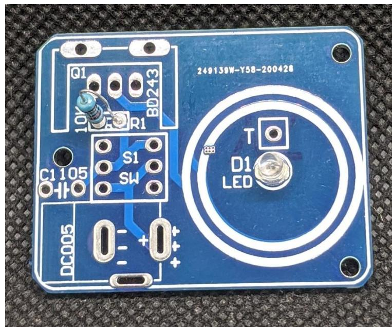
4. Solder the 1uF Capacitor, switch, and DC power jack as shown.
