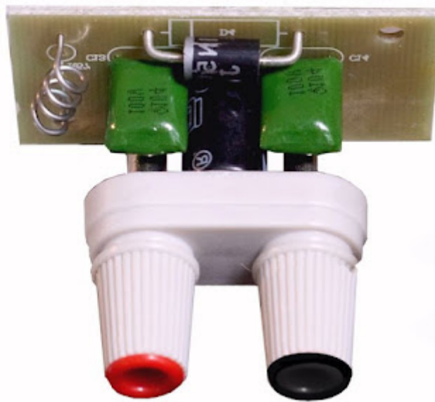
The output PCB with the two 4 mm connectors.
