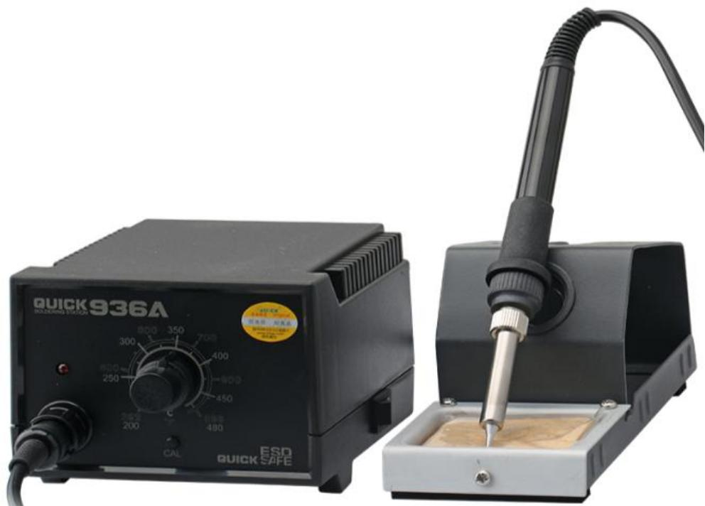
The author uses this kind of soldering iron to weld. The temperature should be about 330 degrees. If it exceeds 350 degrees, it will increase the risk of welded components damaged . If there is no constant temperature soldering iron, it is OK to use 30W low power soldering iron. In short, the welding temperature should not be too high!
