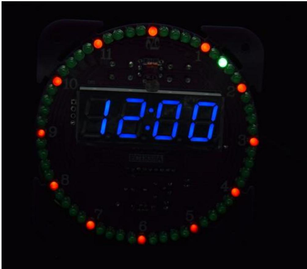
When the display is normal, install batteries on the clock module (note that the positive and negative poles don't be reversed), and then install a housing (if you buy one), it's done!
