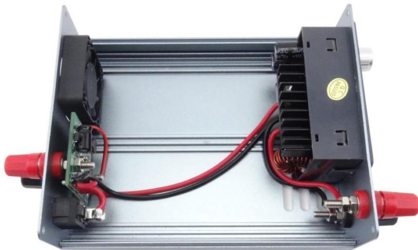
3.4 Extended application extension: you can put 10 pcs 18650 battery in series in the middle on housing to be input power supply. This will be a handheld mobile high-power dc stabilized voltage power supply
