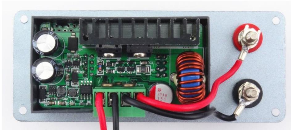
3.2.5 Install the output binding post, and use the output line with cold press connecting terminal to connect input (red is positive above, black is negative below), and screw it tightly
