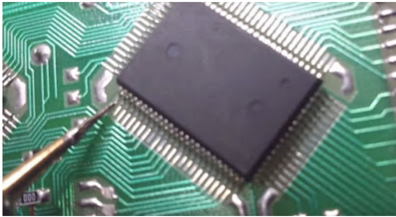
The tip of the soldering iron on one of the pins of a QIP-80A housing.
