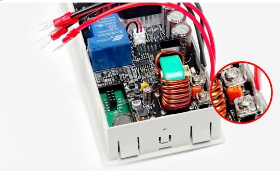
(5) Assemble the switch power supply : Install the switch power supply on the lower board
