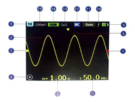
1X/10X mode indicator icon, this must be consistent with the 1X/10X switch setting on the probe handle. If the probe is 1X, then the oscilloscope should also be set to 1X, 1X measures 0~80V, and the maximum tolerance is 800V spike; 10X Measuring 0~800V voltage
