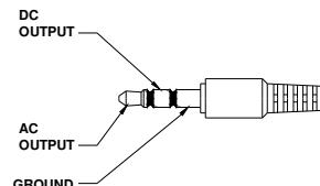
AC:Output voltage: 1Vrms corresponding to each range step.
