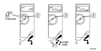
When the meter captures a new input, it beeps and a new reading is displayed.
