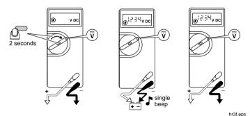
When the meter captures a new input, it beeps and a new reading is displayed. To manually force a new measurement to be held, press .
