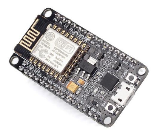
The NodeMcu is an open-source firmware and development kit that helps you to Prototype your IOT product within a few Lua script lines.
